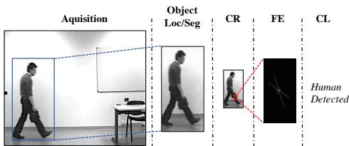
Figure 3: Algorithm demonstration with a real video frame. The system first locates and segments moving object from captured raw image and further compresses the segmented sub-image; then the feature descriptor will be extracted from the compressed object in feature extraction stage (FE) and fed to the template in the last stage for final classification (CL).
