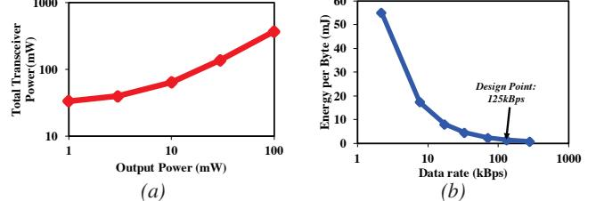
Figure 5: Measured (a) transceiver power vs. output power. (b) energy per byte vs. data rate.
