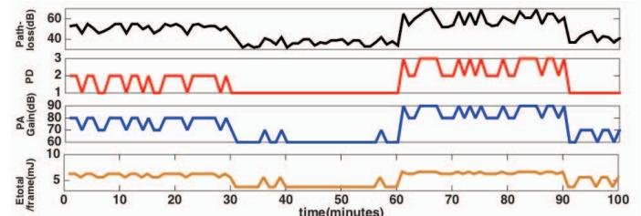
Figure 10: Case study for mobile sensor node with varying path-loss and correspondingly self-optimizing PD, PA gain, and total energy/frame.
