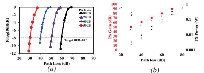
Figure 6: Measured (a) bit-error-rate vs. channel path loss with different PA gain. (b) PA gain and transceiver power vs. path loss for adaptive radio at target  $\text{BER}=10^{-8}$ .
