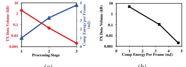
Figure 4: (a) Measured transmission data volume and computation energy vs processing depth. (b) Estimated transmission data volume vs. computation energy.
