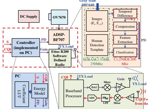
Figure 2: System architecture showing the different hardware components, the image processing pipeline (IPP) and the software defined transceiver. CQI is the channel quality index quantified by path-loss and S is the information content size defined in the following section.
