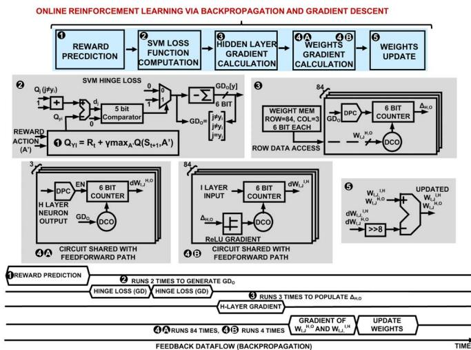
Figure 7.4.3: Flow-chart and corresponding circuit diagrams for online RL via backpropagation and gradient descent.
