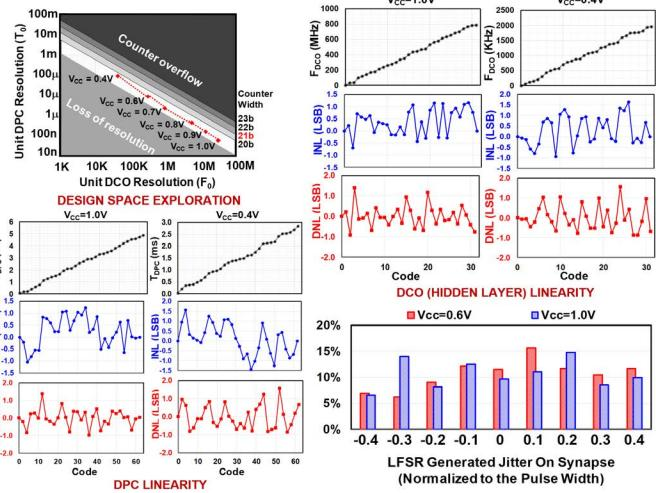
Figure 7.4.4: Design space illustrating measured operating points, measured DCO characteristics, measured DPC characteristics and measured stochasticity generated by the synapses.
