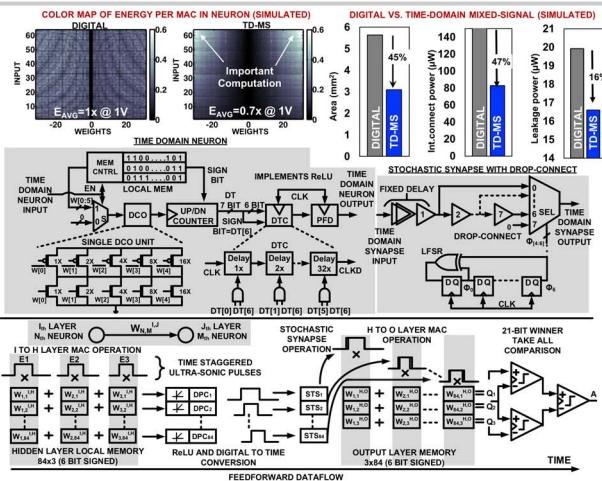
Figure 7.4.2: Comparison of time-domain mixed-signal (TD-MS) design vs. digital implementation, design of TD-MS neuron with ReLU, stochastic synapses and feedforward timing diagram illustrating pipelined data-propagation.
