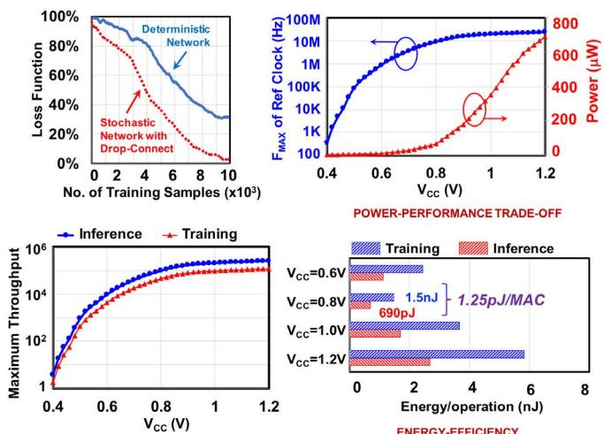
Figure 7.4.5: Role of stochasticity in loss minimization and measured system performance-power trade-offs, illustrating 690 $\mu$ W at peak performance and a worst-case of 1.25pJ/MAC.
