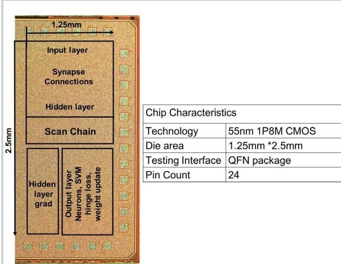
Figure 7.4.7: Die-photo and chip characteristics.
