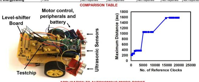
Figure 7.4.6: Comparison table and application to mobile micro-robotics illustrating the use of RL in exploration.
