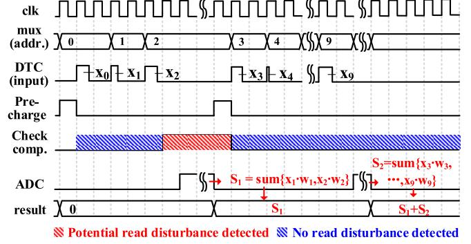
Fig. 8. Timing diagram of in memory vector multiplication process.
