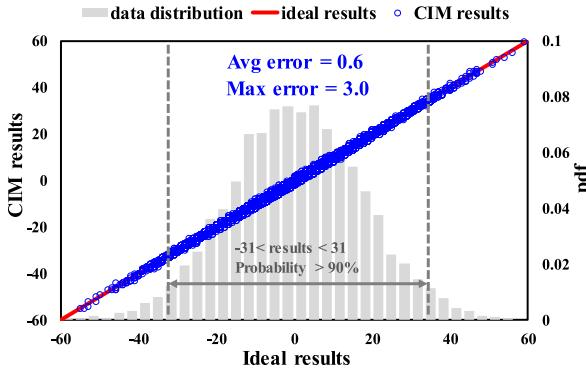
Fig. 12. CIM computing error with uniformly distributed inputs and weights.
