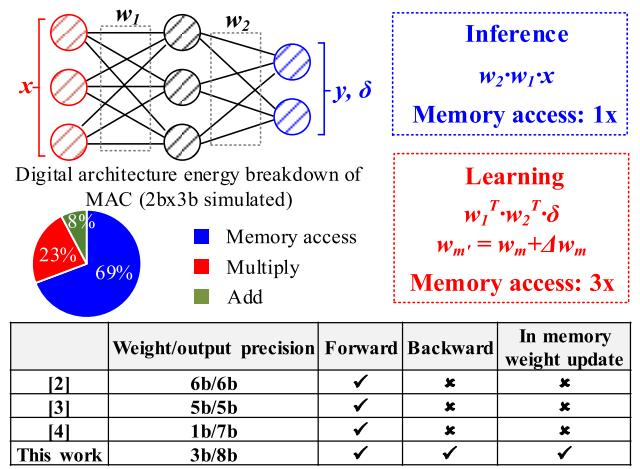
Fig. 1. Inference, learning and memory access of neural networks, digital architecture energy breakdown of MAC, and features of this brief.
