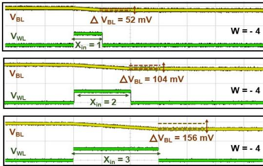
Fig. 11. Oscilloscope capture of BL voltage with varying WL DTC pulse accesses.
