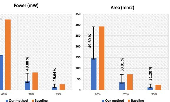
Fig. 5: Measured Power (mW) and area (mm<sup>2</sup>) of the overall system for our proposed and baseline method on VGG-16.
