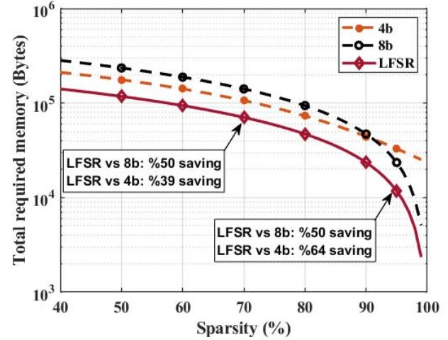
Fig. 4: Total required memory for our method and the baseline method with 4 and 8 bit precision at different levels of sparsity.
