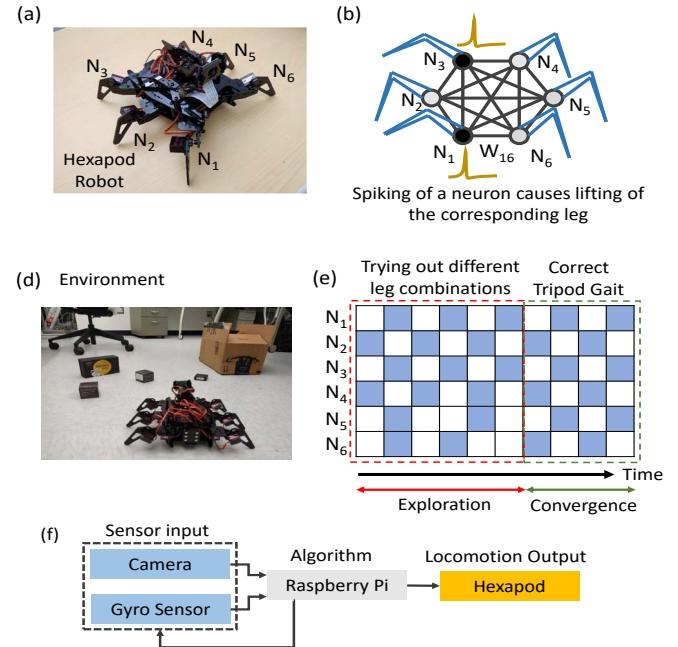
Fig. 1. (a,b) Hexapod robot with labeled neurons for mimicking the CPG. Spiking of a neuron causes motion of the corresponding leg (c) Office environment for demonstration (d) SCPG spiking as the algorithm progresses. The random spiking in the exploration phase gets latched to the correct tripod showing convergence (f) Hardware implementation of the system
