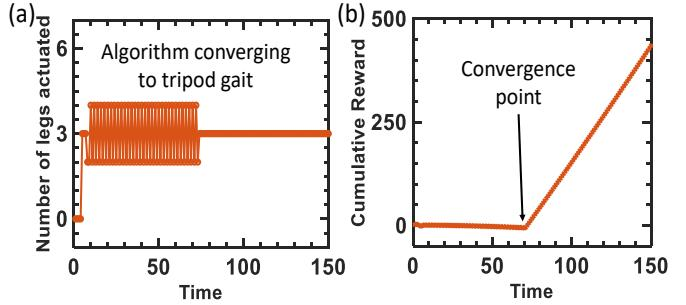
Fig. 3. The number of legs moved at a time instance oscillates around 3 and converges to 3 in a tripod gait resulting in accumulation of high constant reward (b) High positive reward is accumulated with latching to correct gait
