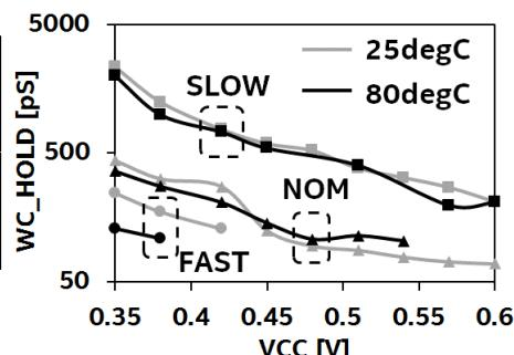
Fig. 11: WC\_HOLD vs  $V_{CC}$  across skew (slow, typical, fast) and temperature (25°C and 80°C)
