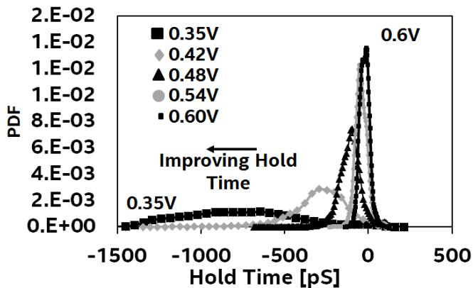
Fig. 5: Probability Density Function (PDF) of hold time with  $V_{CC}$  (0.35V to 0.6V) shows that  $\mu_{HOLD}$  shifts to the left for low voltages
