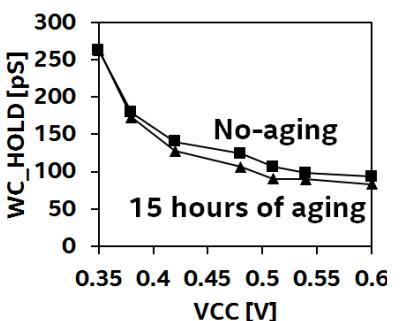
Fig. 12: Aging effect on WC\_HOLD showing minimal impact
