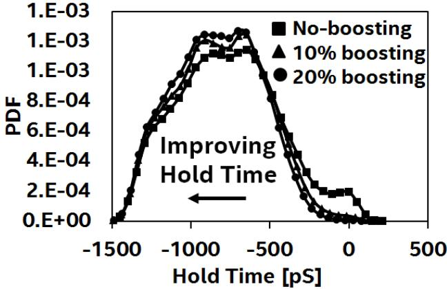
Fig. 13: PDF impact of clock boosting at 0.35V.  $\mu_{\text{HOLD}}$  shifts to the left and  $\sigma_{\text{HOLD}}$  decreases with boosting
