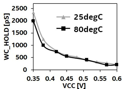
Fig. 9: WC\_HOLD at 25°C and 80°C shows that low temperature is the hold margin limiter
