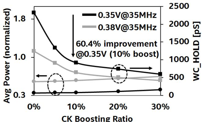
Fig. 15: Power impact of clock boosting
