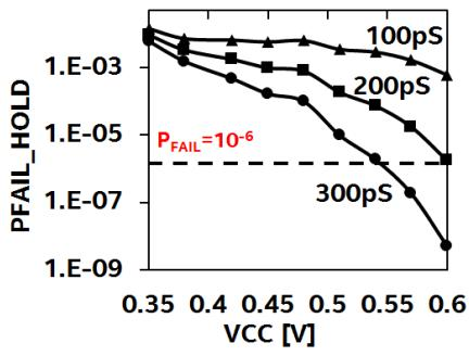
Fig. 7: Probability of min-delay failure ( $P_{FAIL\_HOLD}$ ) vs.  $V_{CC}$  for three different data hold times shows that probability of min-delay failure increases at low voltage
