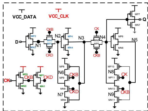
Fig. 1: (a) Schematic of Flip-Flop. Variation in minimum sized transistors MN0, MN1, MP0, and MP1 affects the hold-time and transistors MN2, MN3, MN4, MP2, MP3, and MP4 affects the setup-time. CK is supplied by secondary rail (VCC\_CLK) compared to data-path which is supplied by primary rail (VCC\_DATA)
