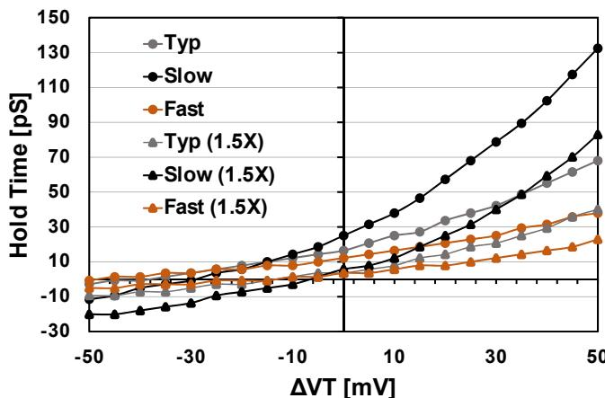
Fig. 1: (b) Hold time as a function of variation in threshold voltage ( $V_T$ ) in transistors in MN0, MN1, MP0 and MP1 across typical (typ), slow and fast process skews at 0.45V, 70degC. Note that sizing (1.5X) of above transistors improves hold-time (simulation)
