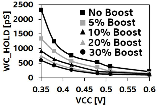
Fig. 14: Clock boosting impact on WC\_HOLD
