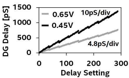
Fig. 3: Delay generator (DG) calibration for 0.45V (larger range) and 0.65V (larger precision)
