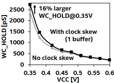
Fig. 8: Worst-case data hold requirement (WC\_HOLD) increases for lower voltages with further increase contributed by clock skew
