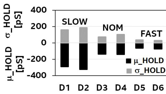
Fig. 10: Die to die variation from 6 dies (2 slow [D1,D2], 2 typical [D3,D4] and 2 fast [D5,D6]) showing variation in  $\mu_{HOLD}$  (negative) and  $\sigma_{HOLD}$  (positive)
