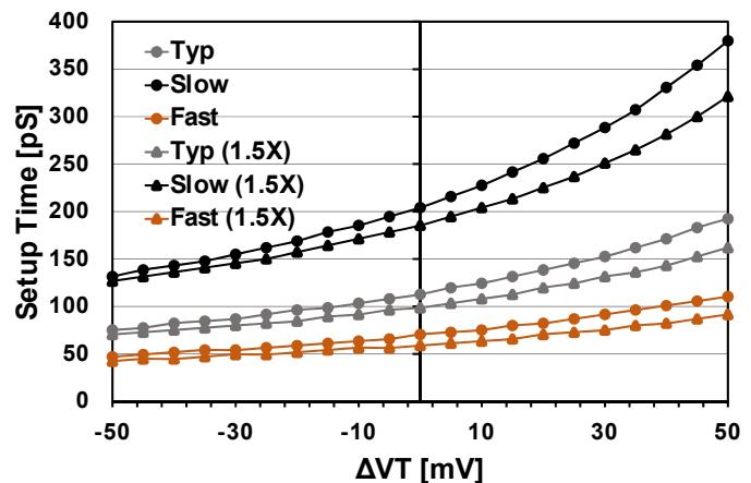
Fig. 1: (c) Setup time as a function of variation in threshold voltage ( $V_T$ ) in transistors in MN2, MN3, MN4, MP2, MP3 and MP4 across typical (typ), slow and fast process skews at 0.45V, 70degC. Note that sizing (1.5X) of above transistors improves setup-time (simulation)
