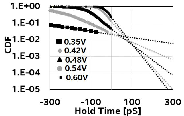
Fig. 6: Cumulative Distribution Function (CDF) of hold time vs.  $V_{CC}$  shows that  $\sigma_{HOLD}$  increases for low voltages
