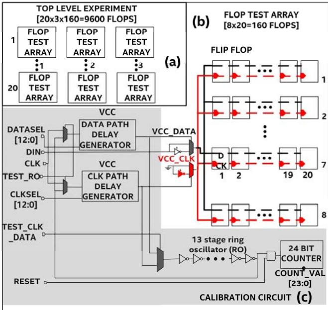
Fig. 2: (a) Test chip block diagram, (b) flip-flop test array, (c) calibration circuit with ring oscillator (RO) and counter
