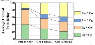
Fig. 1. Elmore Delay Breakdown of top critical paths in High Performance CPU across foundry nodes. Rw, Cw: Wire Resistance & Capacitance, Rg, Cg: Gate Resistance & Capacitance
