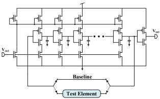
Fig. 2. Calibrating Baseline and Parametric Path Based capacitively loaded current starved RO
