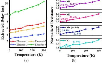
Fig. 4. (a) Extracted Delay from measured frequencies of baseline and parametric ROs across temperature (b) Extracted normalized resistances across temperature (% decrease shown for 100K & 4K).
