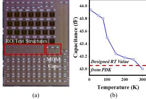
Fig. 3. (a) 22nm FDSOI Chip Photograph showing ROs and MOM Caps (b) Measured MOM Cap across temperature.
