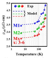
Fig. 6 Fitted Model versus experimental data for  $\rho_{eff}$  of various metal layers.
