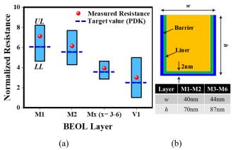
Fig. 5. (a) Measured Resistance of BEOL layers compared with PDK values at Room Temperature. (b) Model of interconnects
