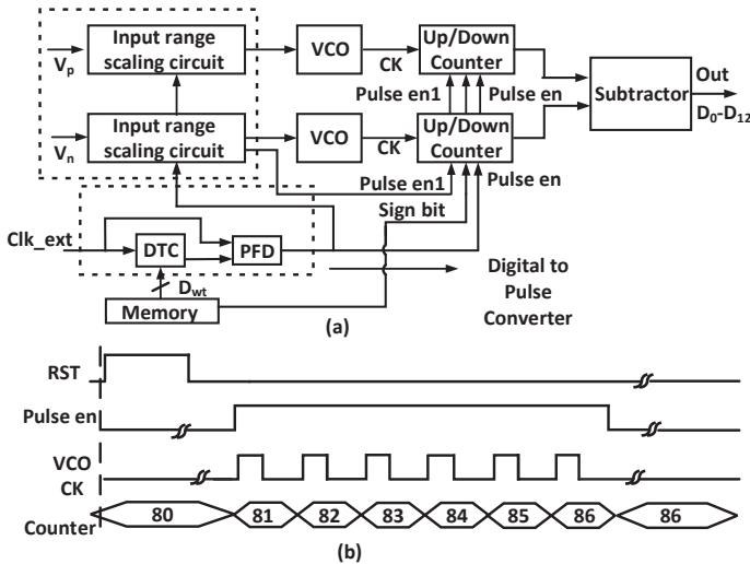
Fig. 3: (a) Proposed pseudo-differential matrix multiplying time-based ADC (b) The corresponding timing diagram
