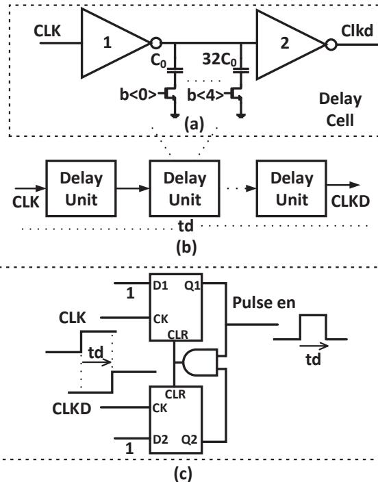
Fig. 6: Digital to pulse converter (DPC) for pulse generation
