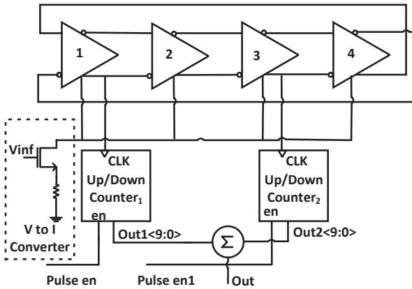
Fig. 4: A single ended VCO along with the output counter
