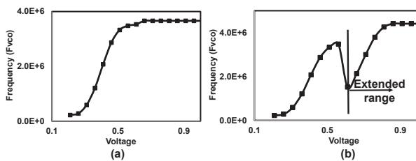
Fig. 9: Measured: (a) Single ended VCO transfer characteristic (b) Folded VCO transfer characteristic with high input range
